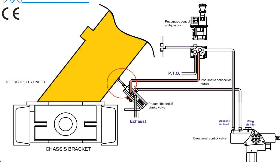
Mounting of the pneumatic end of stroke valve on the tipper must be done as seen on the drawing
